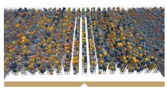
Fig. 2. Five chosen high runners spread in "chaotic" warehouse - colors mean same part number - pallet positions taken from real current WMS. The task = find some clusters.
